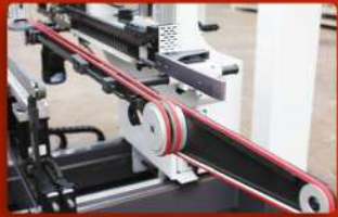
A. Belt type automatic feeding device Stable conveying and more wear-resistant
