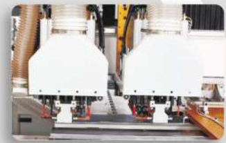
A. One time processing can complete all holes on six sides and double sides grooving for fast and efficient drilling and milling work
