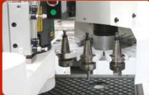
B. The round type tool magazine can hold 12 tools, and based on the principle of proximity to change tools, it is more efficient than milling.
