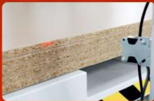
B. With infrared sensor, the lifting platform continuously maintains the set height, and the panel is loaded smoothly
