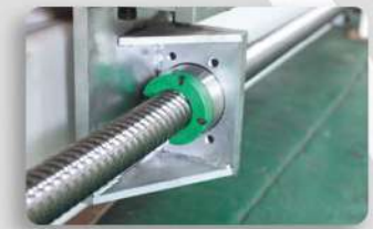
A. Using ball screw drive, after the panel is completed with holes, grooves and other processes, the accuracy of the panel is +0.02mm
