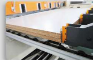
A. Two fingers clamp with plastic cushion, more stable for small panel clamping and feeding
