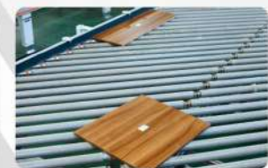
B. Left and right conveying device, through-type processing, shorten panel distance, maximize the utilization of each edge banding machine.
