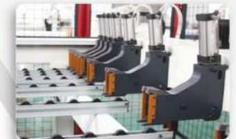
B. Two fingers clamp with plastic cushion, more stable for small panel clamping and feeding
