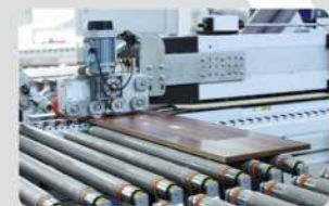
A. Automatic side aligner device, make the panel automatic come to the side, make the edge banding high speed, stable and efficient.
