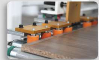
A. Automatically control the side aligning stroke to adapt to the positioning needs of different panel widths
