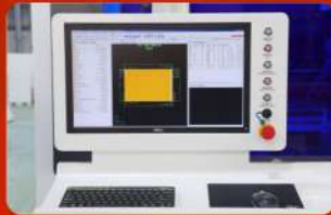
B. The system automatically predicts the size of the left and right worktable panels, and automatically alarms if there is interference to ensure stable processing
