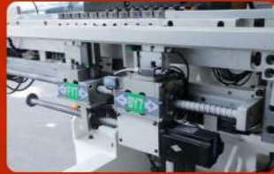
B. Dual servo gripper jaw positioning, precise drilling Precise positioning of the panel during processing, it is not easy to be deflected
