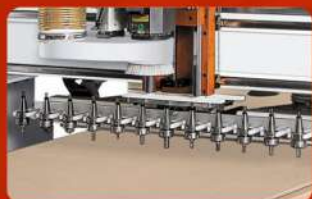
A. Linear type tool magazine with 12 tools, one tool for one craft, automatic tool change without waiting
