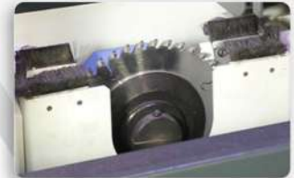
B. Scoring saw can be adjusted front and back, up and down, so that operator can adjust the saw blade better
