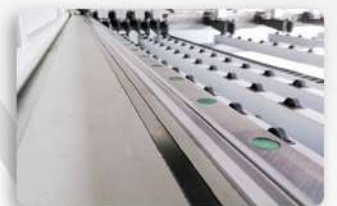
B. Using Taiwan Hiwin precision guide rail, Automatic lubrication, no need to add oil manually
