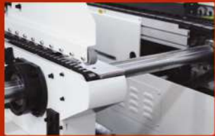
A. Synchronous conveying device, standardized edge banding process, flexible edge banding.
