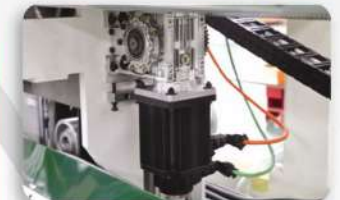
B. Saw carriage speed can reach 120m/min, saw carriage is driven by servo motor, stable and high efficient
