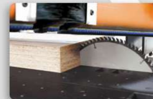
A. Maximum vertical cutting length: 3300mm Maximum horizontal cutting length: 1800mm
