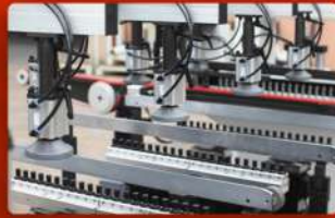
B. Pneumatic pressure , precise drilling, precise positioning of the panel during processing is not easy to be deflected
