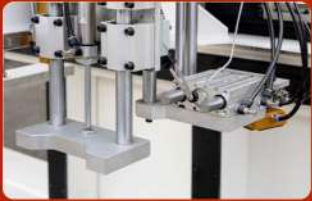
A. Automatic labeling device, intelligently check the width of the panel, and the operation is more user-friendly
