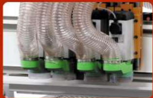
A. Four spindles can be used to process grooving, milling, cutting, and drilling etc
